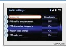
When alternative frequency is set to on, a station providing good reception is automatically selected if current reception worsens.
