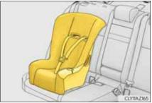
3 Open the anchor bracket cover, latch the hook onto the anchor bracket and tighten the top strap.
