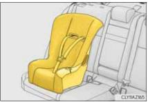
Run the seat belt through the child restraint system and insert the plate into the buckle.
