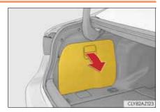
Remove the band and take out the emergency tire puncture repair kit.
