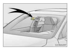
Press the LDA switch to activate the system.
