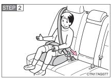
Sit the child in the junior seat. Fit the seat belt to the junior seat according to the manufacturer's instructions and insert the plate into the buckle. Make sure that the belt is not twisted.
